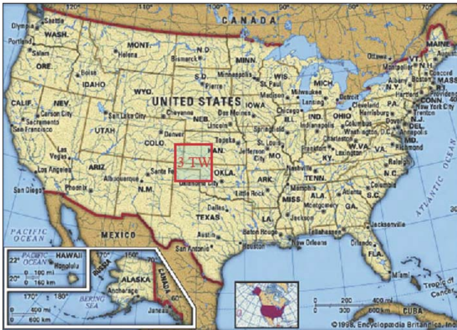
Figure 5. The red square shows the amount of land needed for a solar energy farm operating at 10% efficiency to match the 3 TW of power currently consumed in the United States.
